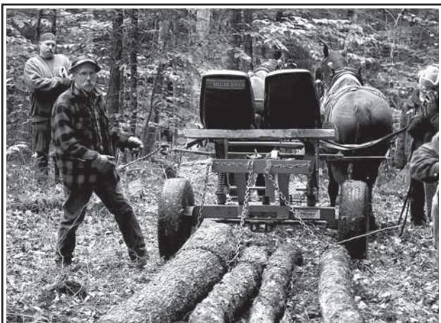
Mark Cowdrey demonstrates the Piggyback Log Arch that he designed to fit on a Pioneer forecart.
