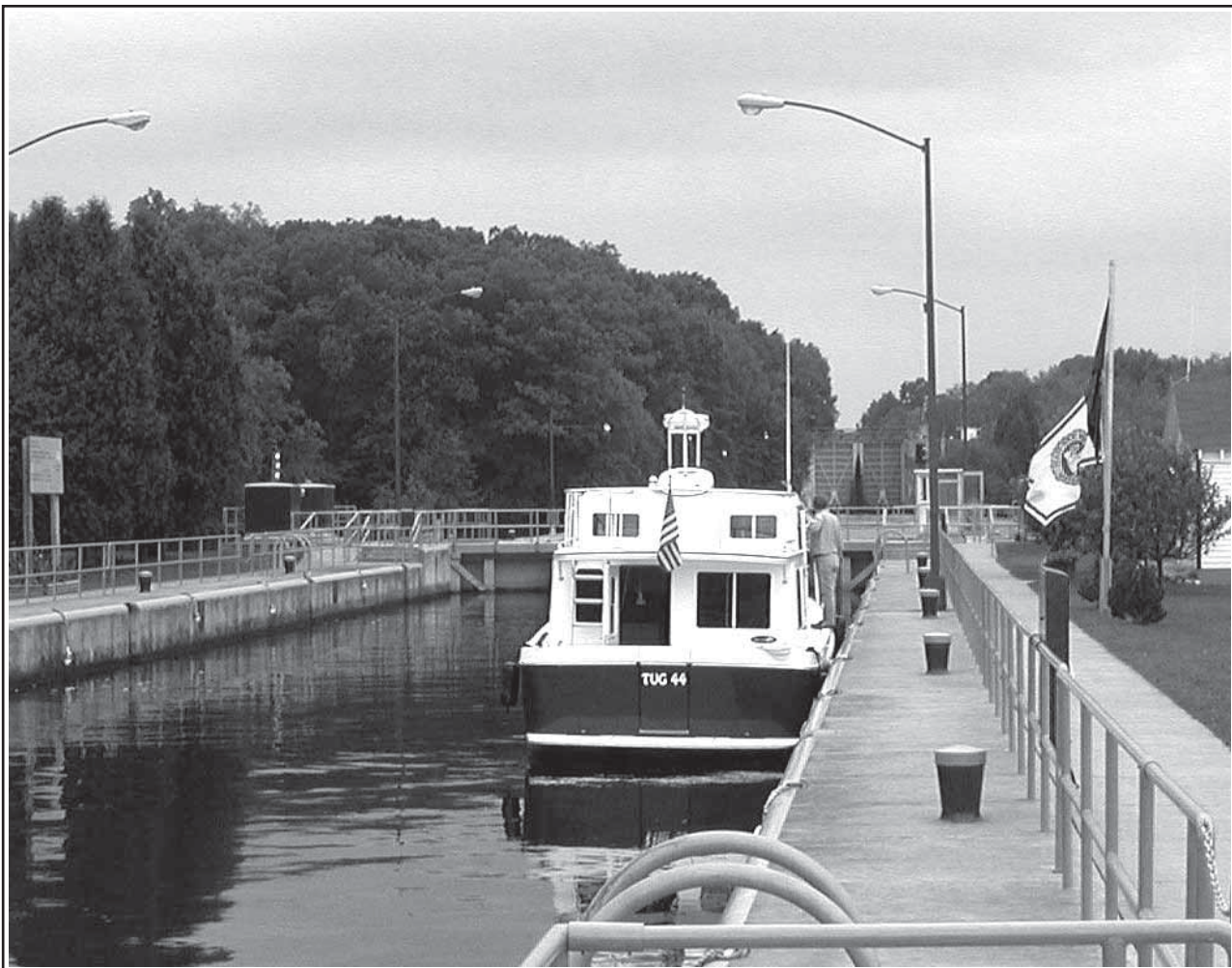
Tug 44 sits in the chamber of Lock E-5 with the lower doors of Lock 6 visible in the background. In the Flight, all 5 locks are right next to each other. photo courtesy of www.tug44.org
