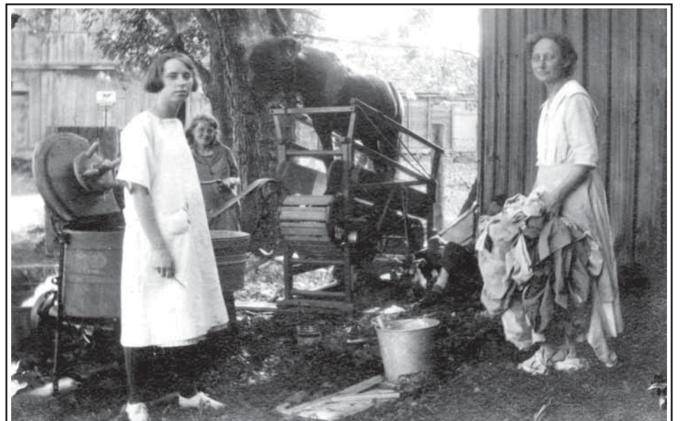
Bertha Doren (on right) and daughter Catherine doing the laundry with a pony-powered rig she made to run the washing machine, Morristown, NY circa 1920.
