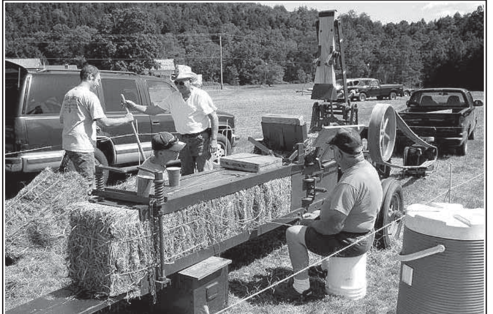
(Left to right) Iain Portalupi of Barre, VT, Shae Martin of Northfield, VT, Ron Bruce of Moretown, VT, and David Newhall of Orange, VT are all working on baling hay using the Vermont Antique Farm Machinery Association's "Turner Stationary Haypress," manufactured in the early 1930s in Statesville, North Carolina. photo by Ted Norman
