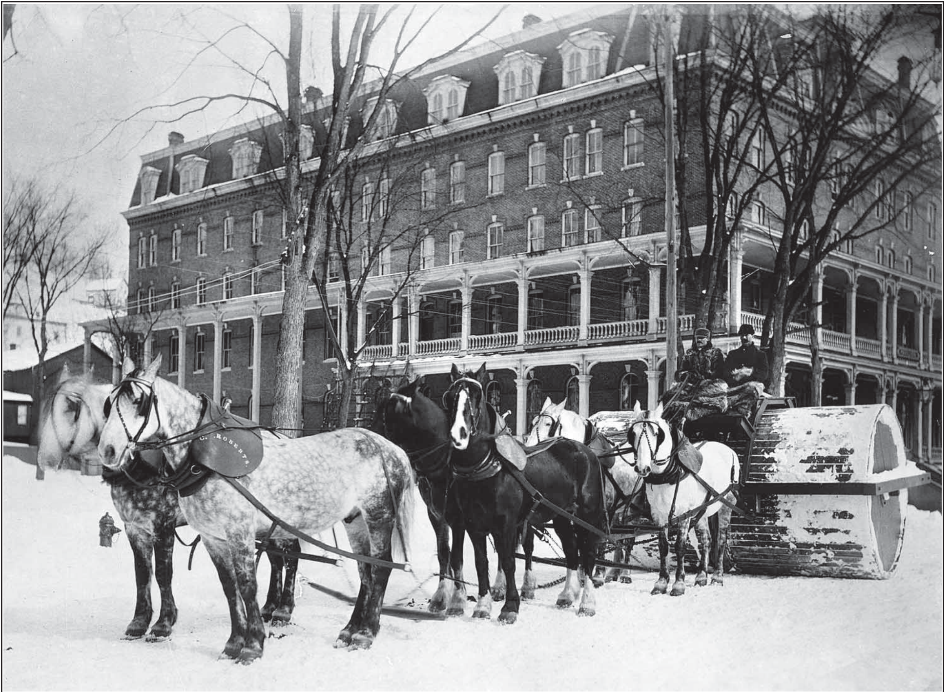
In the late 1800s they rolled the snow instead of plowing it in order to make way for horse-drawn sleds and sleighs. Here is a team of six horses pulling a snow roller on State Street in downtown Montpelier, VT in front of the Pavilion Hotel. photo courtesy of Vermont Historical Society
